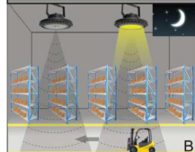
If the ambient light is dimmer than the preset ambient luminance threshold (can also be reset via controller) and the sensor detects some moving object, the light will be on automatically and reach the preset luminance of active level (can also be reset via controller).
