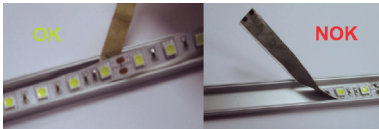
Image 3. Fitting the LED strip while removing the protective adhesive
