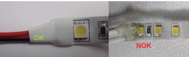
Image 8. Protection of the LED strip - connector cable using heat-shrink material
