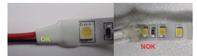
Image 8. Protection of the LED strip - connector cable using heat-shrink material
