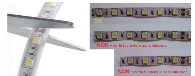
Image 5. LED strip cutting OK y NOK
