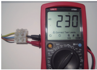
Between neutral and earth 0V.
